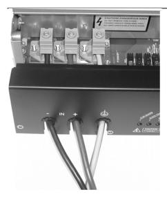
Figure 1. Cable connection for 24V and 48V inputs.
