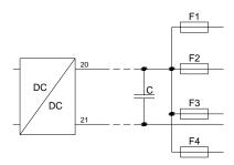
Figure 4. Connecting multiple loads.
