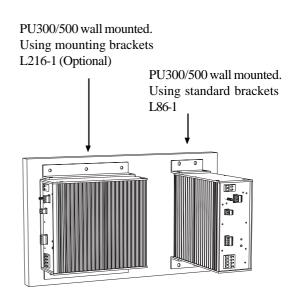
Figure 3. Wall and chassis chassis mount
